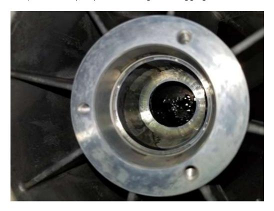
10) Lubricate first main pump bearing.
