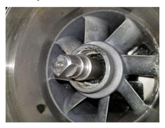
7) Remove new shaft and rear bearing from upgrade kit. Press the bearing on the back as shown below. Please make sure to only press down on the inner race, pushing on the outer race will damage the bearing.
