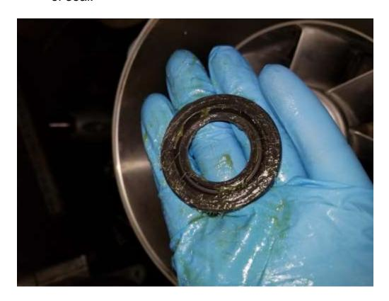
18) Pack grease on top of next seal, and repeat. Be careful not to damage the seal.
