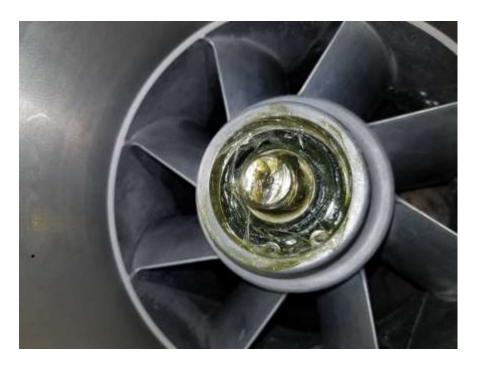
23) Hold back of impeller shaft in vice as shown.
