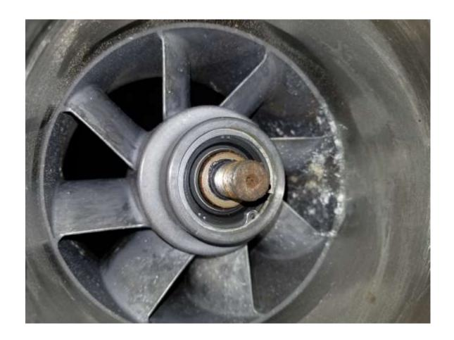
3) Pull up on impeller shaft to remove shaft from housing. If shaft is very tight, you can use a rubber mallet to hit it out. Do not use a metal hammer!
