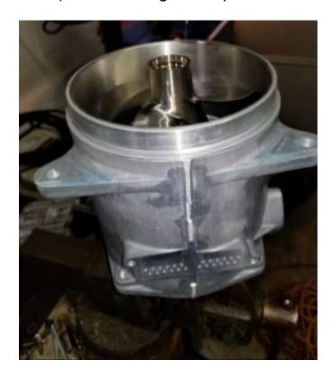
25) Insert spline tool and tighten to 110 ft.lb.
