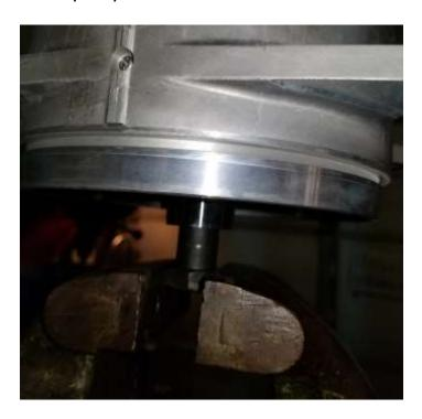
27) Install supplied high strength nut, torque to 72 ft.lb. No locking agent or grease necessary here.
