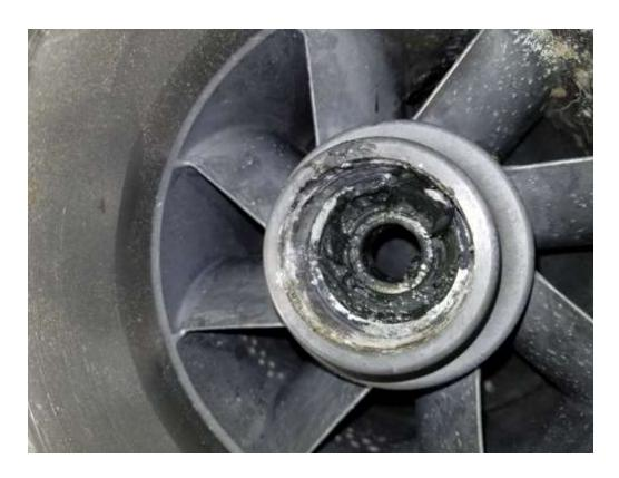
6) Take old shaft and insert it upside down as shown below. Push bearing out.
