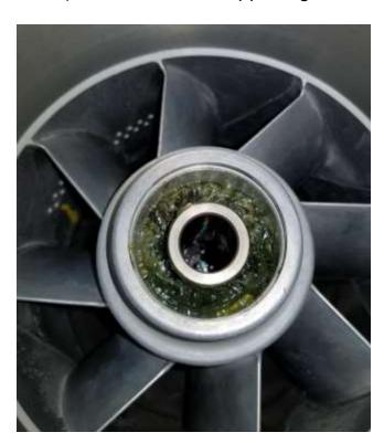
17) Install first seal. Spring always faces up! You can use a large socket for this, but be careful only to push on outer portion of seal.
