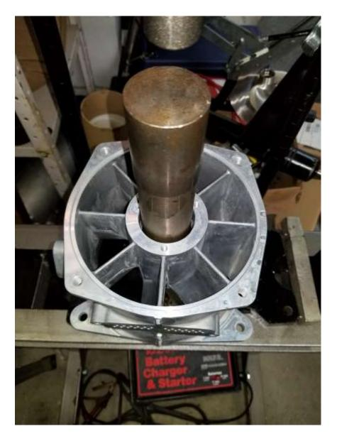
13) Press bearing in until it bottoms out. We recommend a mechanical press over hydraulic.
