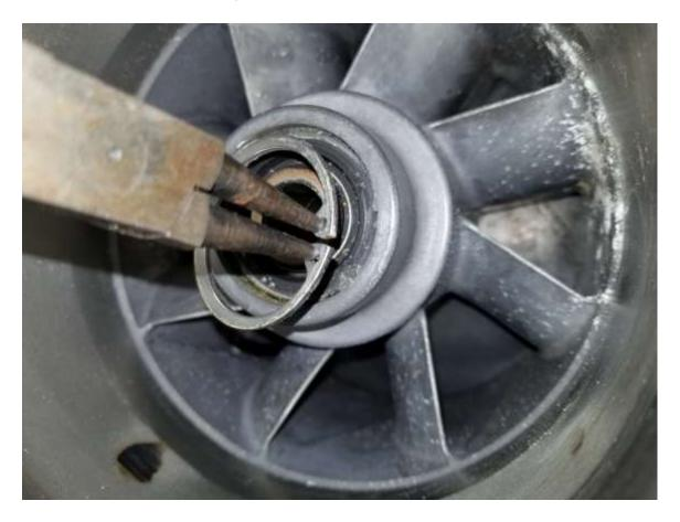
5) Using a rigid screw driver, pry the old seals out from the inner lip. DO NOT PRY ON THE OUTER SURFACE!
