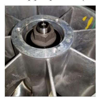
28) Install cones, trim seal and hardware. Please follow the torque specs below.
