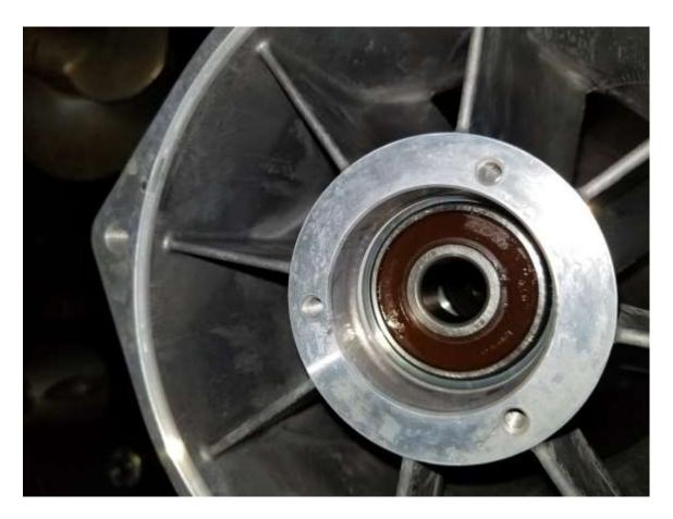
12) Insert bearing installation tool. Remember, you may only press on the outer race or you risk damaging the bearing.
